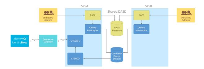
When a transaction is issued by IdentityIQ, it is executed by the Connector Transaction Server (CS) running on the primary system, and the appropriate updates are made to the RACF database.
