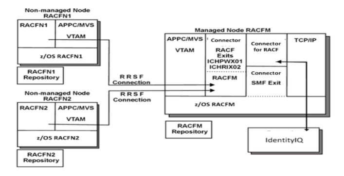
In the previous example, some RACF events on non-managed nodes are synchronized with RACF on the managed node and are consequently intercepted by Connector for RACF on the managed node.
