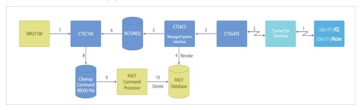
When the Delay parameter is used in a delete request, IdentityIQ instructs Connector not to perform the delete request immediately, but to queue it for delayed processing [1].
